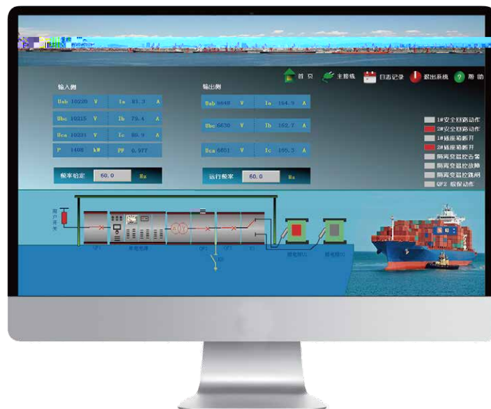
Shore Power Monitoring System
